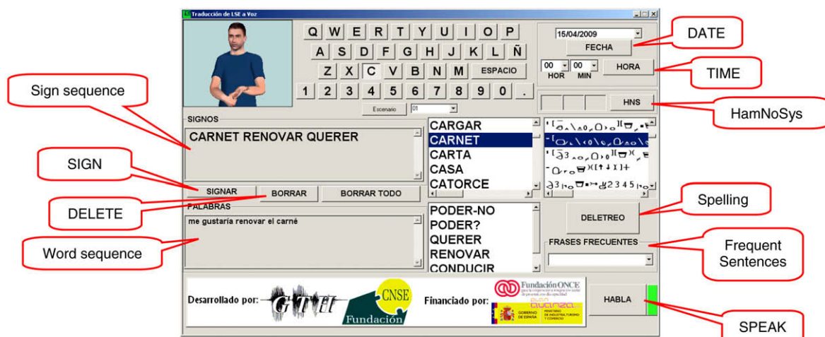
Fig. 11. Advanced visual interface for sign sequence specification. The sign sequence CARNET RENOVAR QUERER (LICENCE TO_RENEW TO_WANT) is translated into "me gustaría renovar el carné (I'd like to renew the driving licence).
